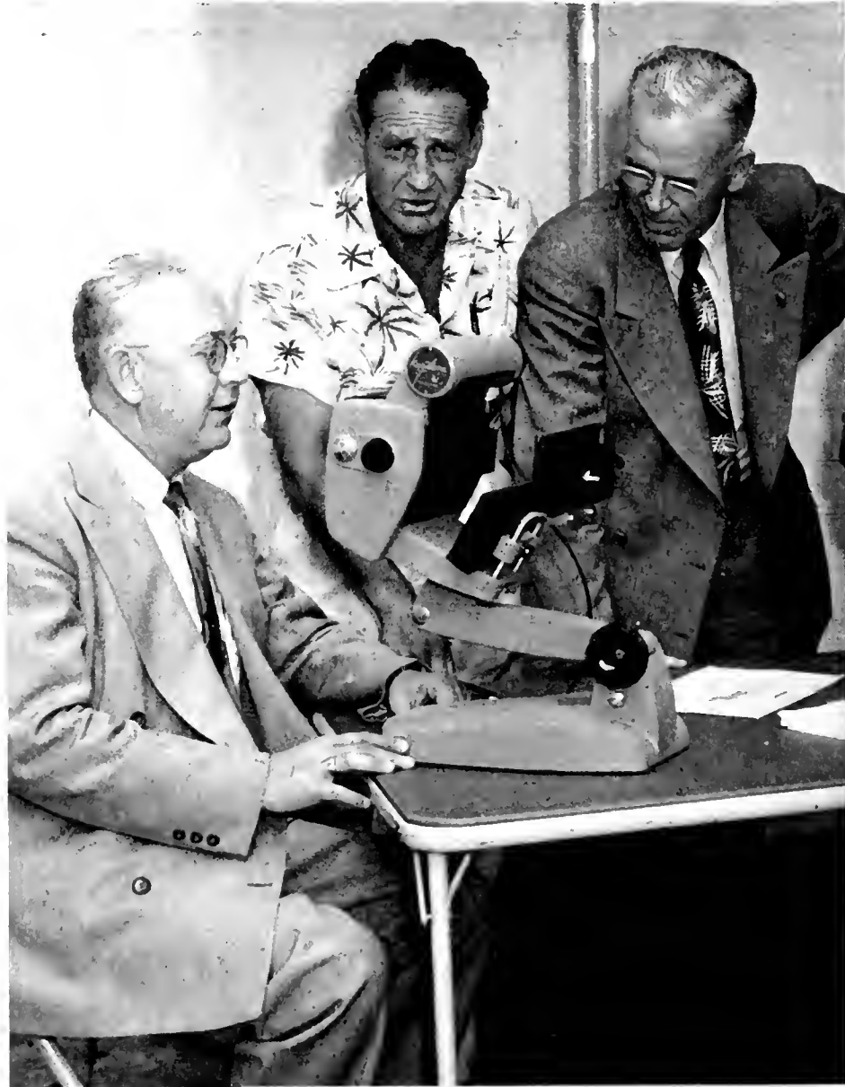
Testing vision by telebinocular. This instrument tests a driver's visual acuity, depth perception, muscular imbalance and his color vision. LEFT TO RIGHT: Paul O. Harding, Assistant State Highway Engineer, District VII; Carroll T. Berry, Associate, Safety Section; W. L. Fahey, District Engineer, District VII.
